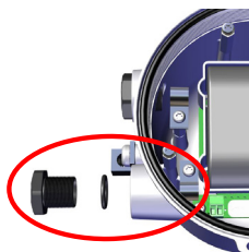
Remove plug & o-ring. Insert cable gland/strain relief. Feed cable through cable gland.
